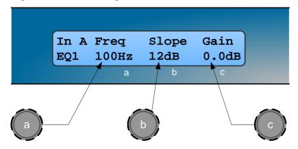
Knob A: Frequency, 10.0Hz to 25.6kHz in variable steps
