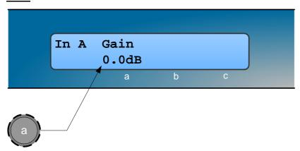
Knob A: Gain, adjustable in 0.2dB steps from –80 dB to +20dB
