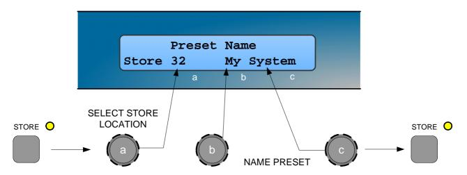
The user can overwrite non-protected Presets only; if an attempt is made to save a Preset in a location already occupied by a Factory Preset a 'LOCKED PRESET' message is displayed.
