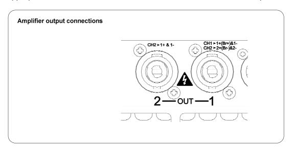
The Speakon<sup>TM</sup> connector for amplifier channel 1 carries the output for amplifier channels 1 and 2. In addition this connector can also be used if the pair of amplifier channels is being operated in bridged mode.
