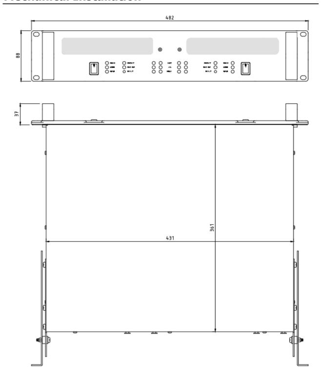
The XiB DSP amplifier system is designed to be mounted in a standard 19" rack enclosure. Where the amplifier is used in a fixed installation, it is possible to use only the front panel 19" rack mounting holes to mount it in a standard rack enclosure. If the amplifier is
