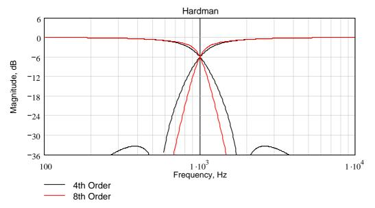
The following plots show the magnitude response (frequency response) characteristics of the various equalisation filters available within the XiB. These are all shown at a c frequency of 1kHz.
