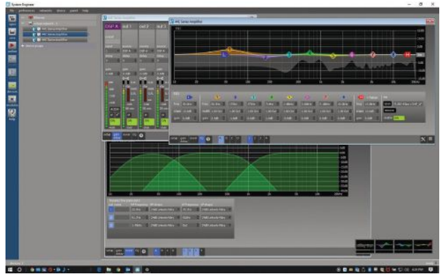
A screenshot of the System Engineer app for setting up, controlling, and monitoring all Linea products.
