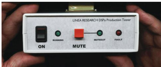
Linea makes all of its own test equipment for production, and this is one example.
